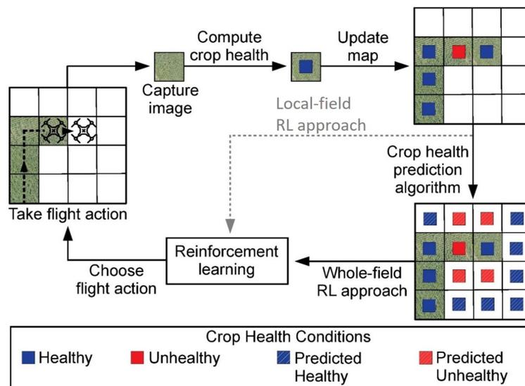
**Figure 2.** Fully autonomous aerial crop scouting uses RL to decide flight actions and covers only a fraction of the field.
