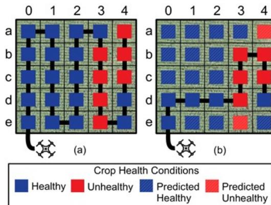
**Figure 1.** (a) Exhaustive scouting of a field wherein UAS visits all zones in a grid fashion and crop conditions are classified as healthy and unhealthy, and (b) RL based fully autonomous aerial scouting wherein UAS visits over a fraction of a field (e.g., 8 areas) and predict crop conditions for unvisited areas.
